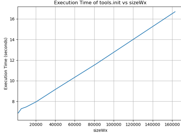
Figure 5. Execution time of the insertion procedure compared to the number of watermarked parameters N .
